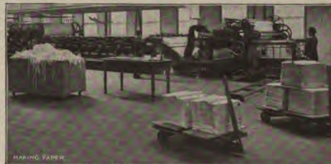
Making paper at Portland, Maine: Rags and wood fiber are ground into pulp. This is pressed into sheets by passing through many iron rollers which dry and finish it.
